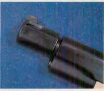
ABOVE: Bushing is visible between Plaxco Compensator and slide. Otherwise, compensator looks like slide extension.
